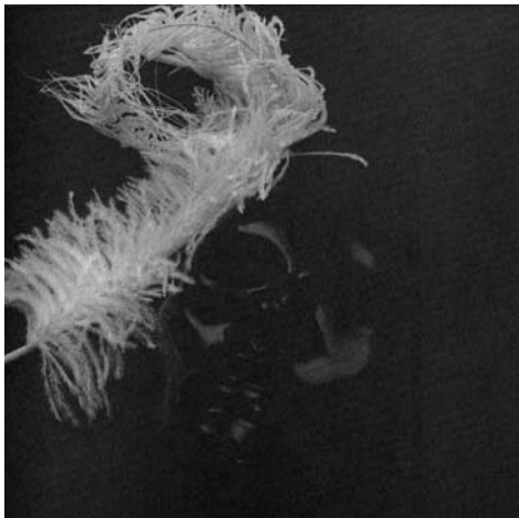
3.14 A polarizer over the camera lens blocks the polarized direct reflection. Only the feather, which gives off diffuse reflection, is easily visible.
